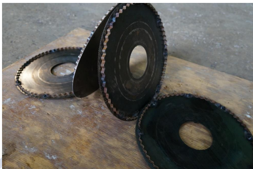
3-rasm. Arraga qistirmalarni payvandlash.
